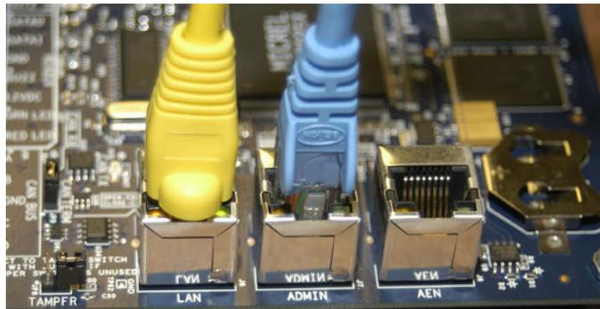
Figure 4: **ACS5000** - Connect Main Board to LAN
