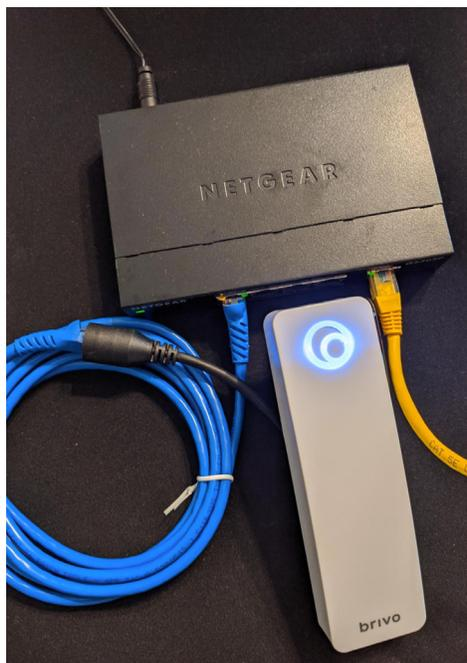
Figure 40: **ACS100** - Connect laptop to control panel through switch
