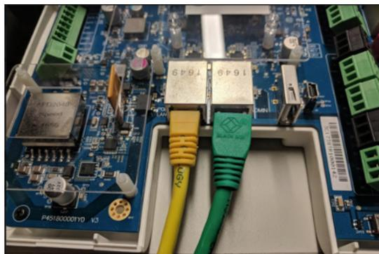
Figure 6: **ACS300** - Connect Main Board to LAN
