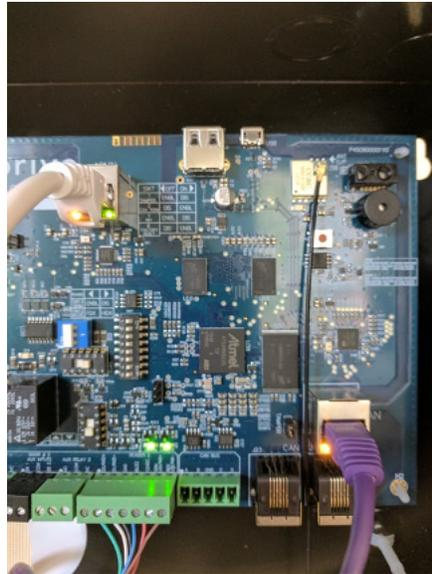
Figure 5: **ACS6000** - Connect Main Board to LAN
