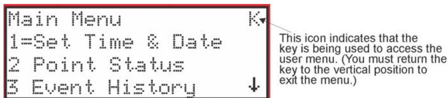
Figure 8-3 Using a Key to Access the Main Menu
