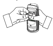
Figure 14. Pulling the battery tab
