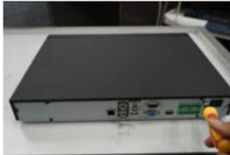
Figure B-1 Removing the NVR Cover
