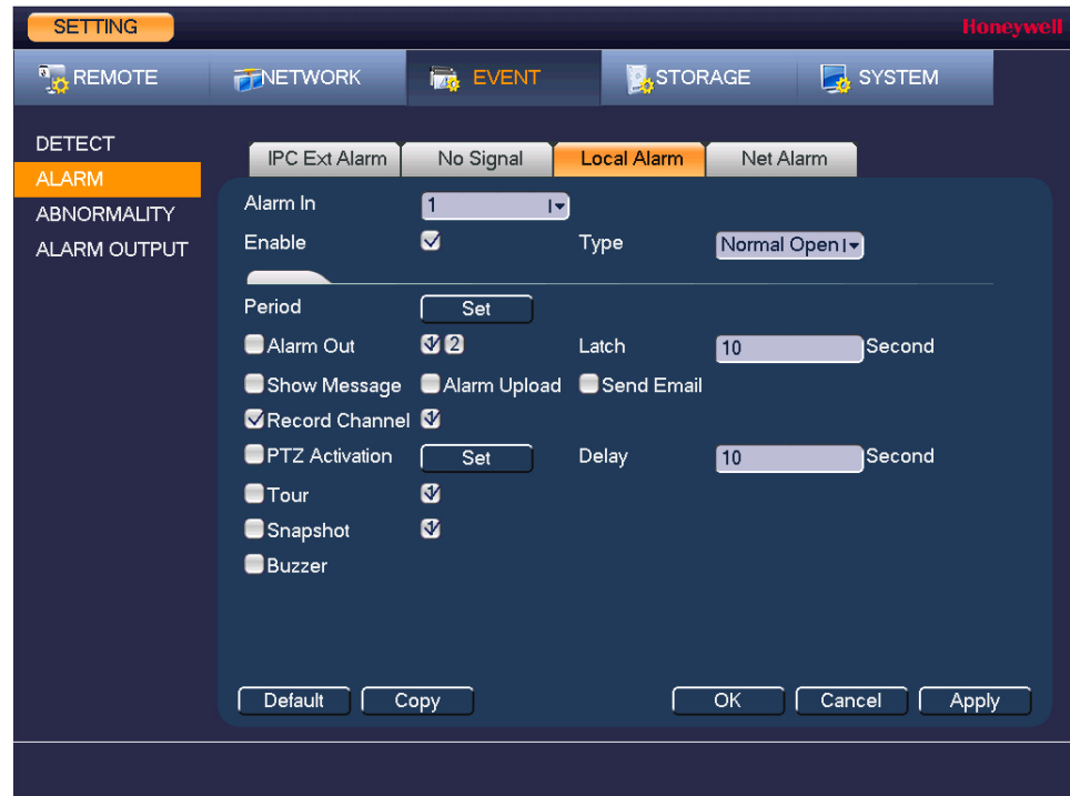
Figure 8-12 Event - Local Alarm Configuration Tab
