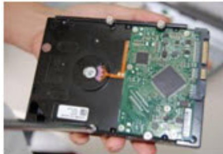
Figure B-2 Loosening the Four Screws in the HDD Housing
