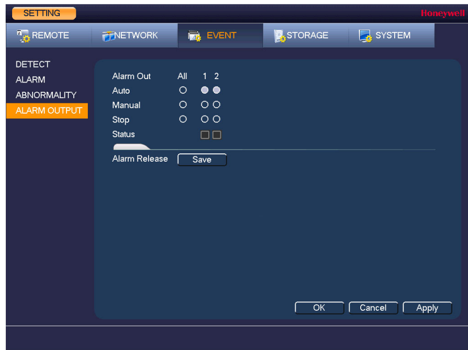
Figure 8-14 Alarm Output Configuration Tab
