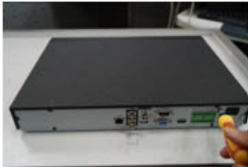
Figure B-7 Securing the NVR Cover
