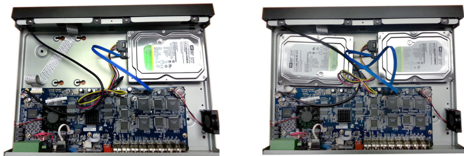
Figure B-8 Installing a Second HDD
