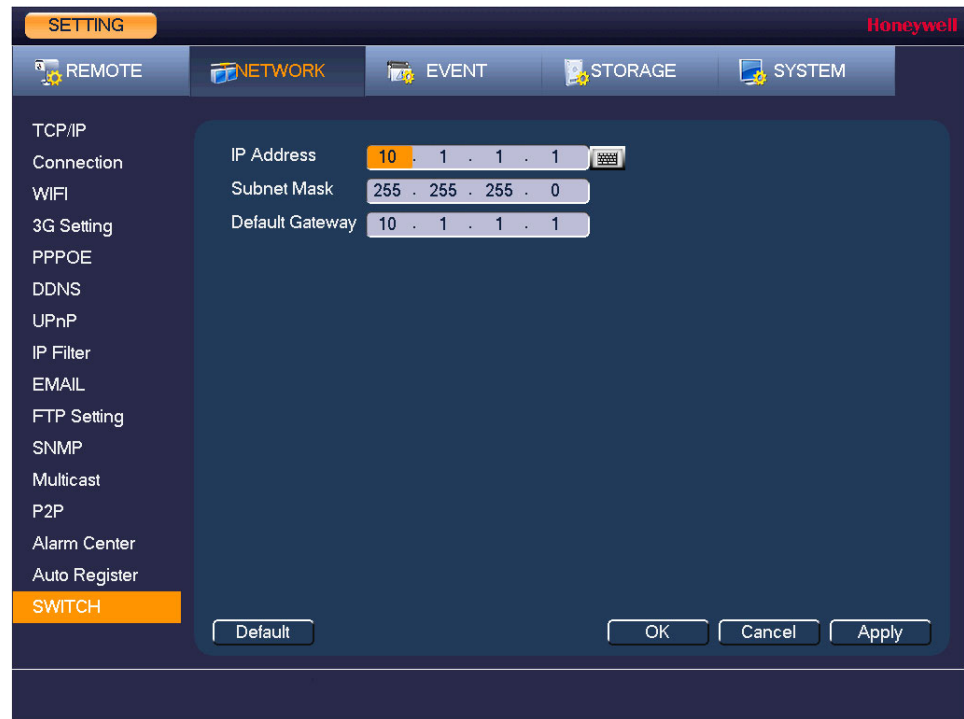
Figure 7-14 Network Switch Settings Window
