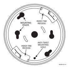
Secure the sensor to the mounting base by aligning the sensor's index tabs to the index tab recesses on the mounting base. While pushing in, turn the sensor clockwise until it locks. DO NOT touch the metal disc.
