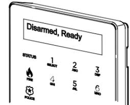
1. At the Smart Controller, enter Programming mode and follow the control's instructions to enter keypad enrollment mode (Program > RF Keypad > Add New > Serial No.).
