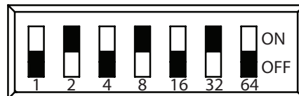
FIGURE 10: Enlarged View of PAD Device with Dip Switch Setting Addressed
