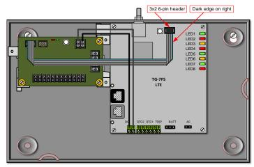
Connect ribbon cable (provided) from the connector on TG-PEM labeled "TO HOST" to the 3x2 6-pin header on the TG-7 series board as shown. The dark color edge of the ribbon cable should be oriented away from the antenna of the TG-7 or TG-7FS.
