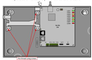
Use the three provided mounting screws to secure the TG-PEM board onto the bracket.
