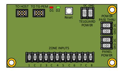
Note: At power-up, both LEDs will be on for 3 seconds then off for 3 seconds.
