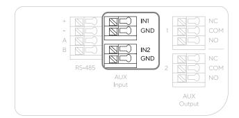
With the AC41's AUX inputs you can hook up devices such as intercoms and buttons into the auxiliary cassette of the AC41, and all associated unlock events will be logged in Command.
