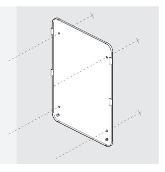
Place the sheet metal enclosure over and onto the mounting plate tabs.
