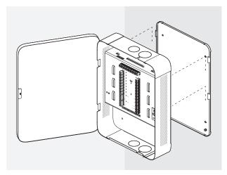
Fasten the two security torx screws to secure the enclosure to the mounting plate.
