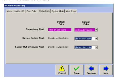
The Status Color window allows Supervisory, Device Testing, and Facility out of Service alerts to be customized.
