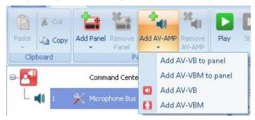
Once the amplifier is added, clicking within the amplifier's text location allows the user to define a custom label for the amplifier (32 characters). In our example we have labeled the amplifier as a Floor/Area Amplifier.
