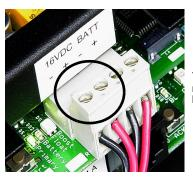
Test voltage from the power supply to the BT-X by placing multimeter leads on these screwheads after removing the battery leads.
