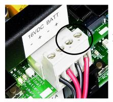
Test voltage from the charger to the battery by placing the multimeter leads on these screw heads.
