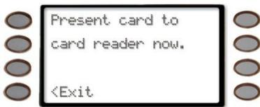
Present the card to the reader to continue or press the **<Exit** soft key to exit out of this function and return the display to idle text.
