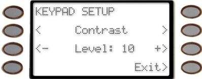
Each of these selections have <- **Level** +> soft keys on either side of the display that allows you to increase (+) or decrease (-) the setting being displayed. The High and Low Brightness are associated to Command 49's Bright Display and Dim Display settings.
