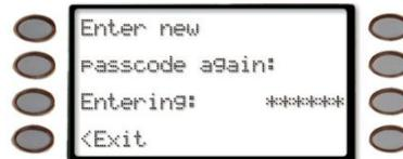
The passcode is shown as asterisks (\*) when entered and advance from the right side of the display to the left until all six passcode digits are entered.
