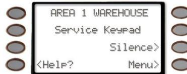
Indicates that a command center, other than the one displaying the message, is in a trouble condition. Notify your security company.
