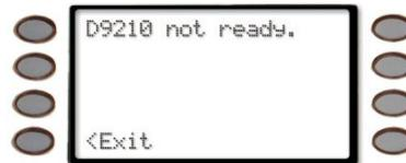
If 20 seconds elapse without pressing a key the display returns to idle text. Pressing the **<Exit** soft key exits out of this function and returns the display to the main **Add / Change User** display.
