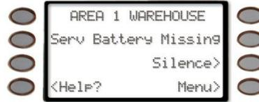
Indicates the security system's battery is disconnected or shorted.
