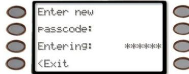
The passcode is shown as asterisks (\*) when entered and advance from the right side of the display to the left until all passcode digits are entered.
