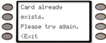
If 20 seconds elapse without pressing a key returns the display to idle text. Pressing the **<Exit** soft key exits out of this function and returns the display to the main **Add / Change User** display.
