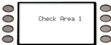
If there is a faulted point in more than one area and the system is being armed, the display will prompt **Check Area 1 3** meaning there are faulted points in Areas 1 and 3.
