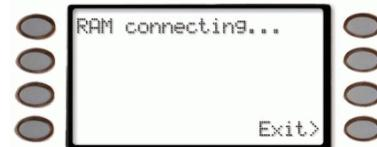
10. The security system will now disconnect telephones sharing its telephone line during the remote programming session. Hang up the telephone now.
