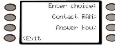
16. Press the **Contact RAM**> soft key to specify the connection method to RAM.
