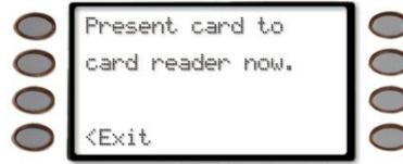
Pressing the **<Exit** soft key exits out of this function and returns the display to idle text.
