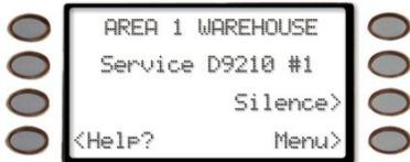
Indicates that one of the D9210 Access Control Modules (possible of 8 total) connected to the panel has encountered a problem. Contact your security company.
