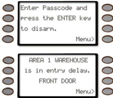
The command center emits a tweedle tone and alternates between **Enter Passcode and press the ENTER key to disarm** and **AREA 1 WAREHOUSE is in entry delay**. (AREA 1 WAREHOUSE is used as an example.)
