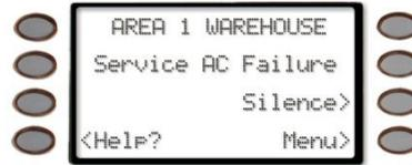
Indicates that AC power to the security system is interrupted. Check the plug-in transformer and circuit breaker. Entering COMMAND 4 silences the trouble buzz. The display clears when AC power returns.
