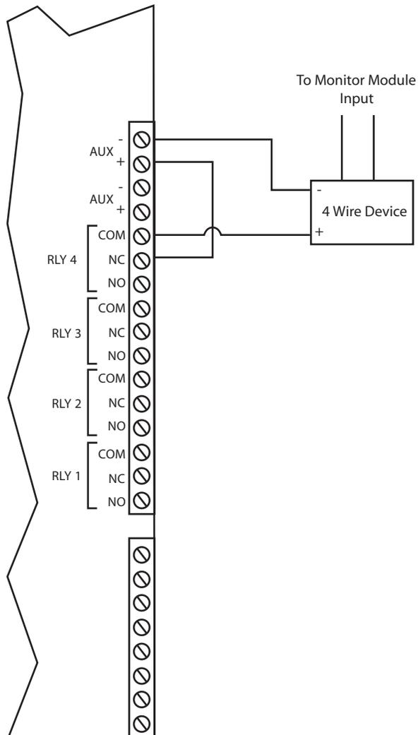
Figure 1: Four Wire Device Wiring (Typical)
