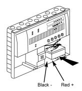
Figure 3. Battery Connection location
