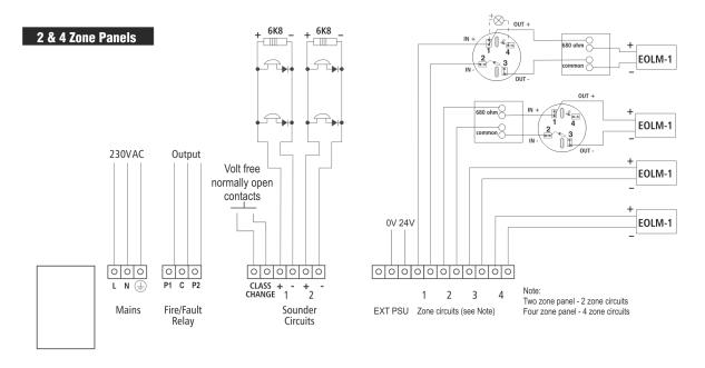
Figure 5. Wiring connection drawing
