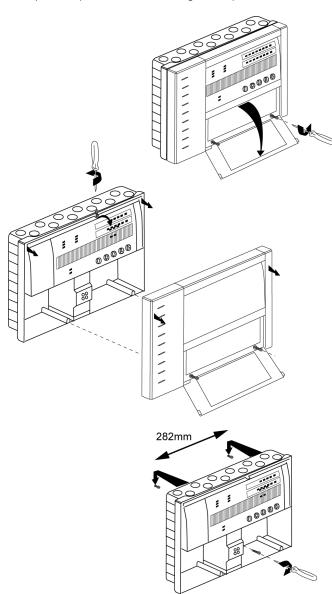
Figure 1. Panel installation
